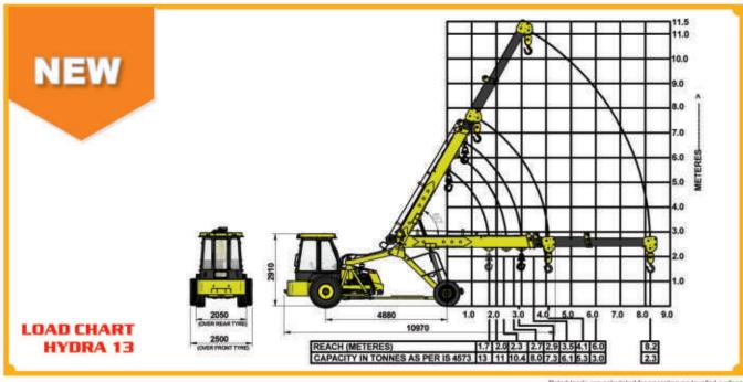
Rated loads are calculated for operation on levelled surface.
